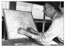
Lookout men used firefinder equipment to most accurately pinpoint locations of possible wildfires. The lookouts would plot the direction of the smoke on a map and contact two other adjacent towers to receive the smoke direction from their locations. With these three plots, they triangulated the approximate smoke location and dispatched fire suppression crews.
