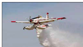
TetraKO testing at TEEX included three separate trials of TetraKO released from the Fire Boss aircraft tank, including a Level 1 coverage drop, a Level 3 coverage drop and, finally, a full Salvo coverage drop. TetraKO clings to trees, bushes and grasses and won't fall to the ground, and can be applied to wildfires from air, truck or backpack.
